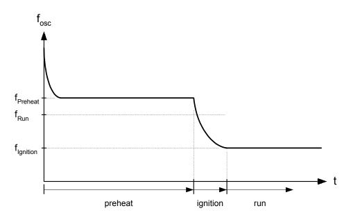
Fig. 6.1: Oscillator frequency versus time, Normal operating conditions
