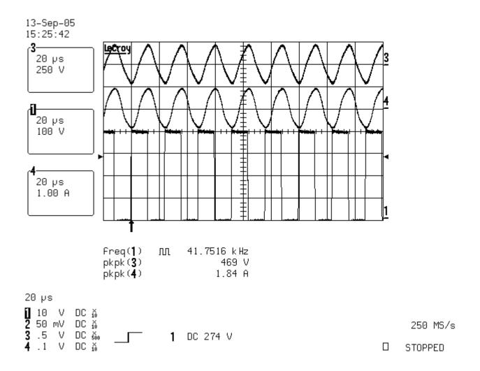
Fig. 6.4 Lamp voltage (CH3), lamp current (CH4) and Half Bridge VS voltage (CH1) during normal operation
